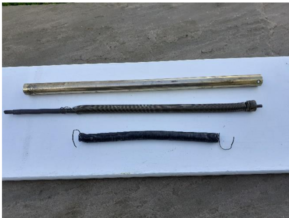
The new spring attached to the mechanism, which is housed in the tube. The original spring sits below. (photo L. Rodway)
