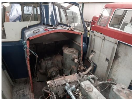
Above left: work in progress stripping out DH16's engine bay ready for transmission removal. 19/3/21
